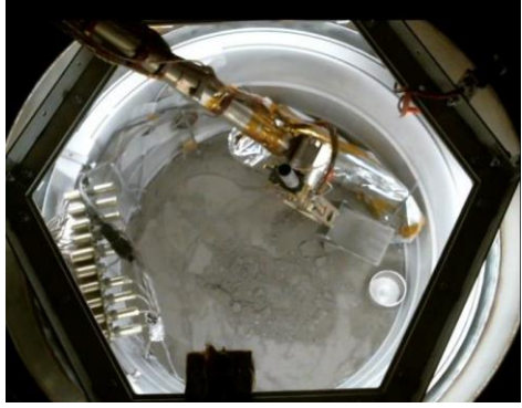
Figure 2. The concept of cryogenic vacuum chamber used for the robotic arm tests (LEFT). The photo of robotic arm operations in cryogenic vacuum chamber: excavation, sample acquisition and delivery to the special container (RIGHT).
